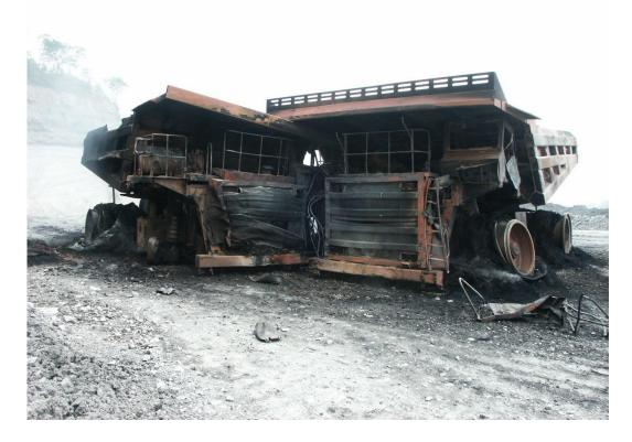
On August 10, 2004, an accident occurred at approximately 1:15 a.m. when a 789 hauler was traveling up an approximate 4% grade. While negotiating a right switchback, the 789 hauler was struck in the left fron side by a 785 hauler traveling downgrade in the switchback. This collision resulted in an immediate fire in the engine compartment area of the 789 hauler resulting in loss of both haulers.
