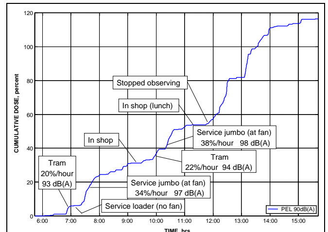
Figure 8. Cumulative dose plot of a service mechanic's work shift [5:45 to 15:45].
