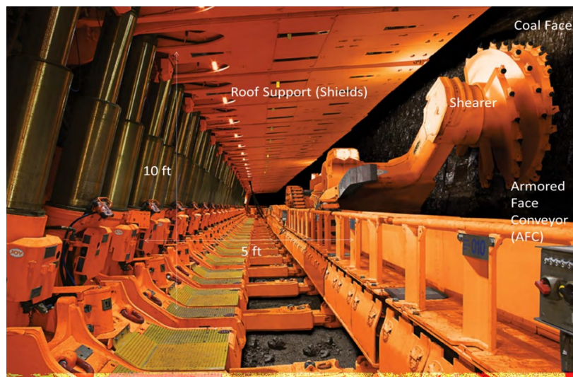
Figure 1.2: Typical longwall system (Joy Global, 2014)
