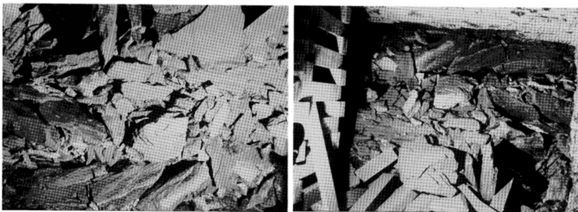
Figure 3.15: Gob at two coal mines in eastern Kentucky (Pappas and Mark, 1993a)
