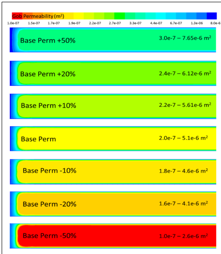
Figure 5.7: Contours of the gob permeability variation used for sensitivity analysis
