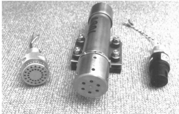
Figure 3.9: Machine-mounted sensor head (Taylor, et al. 2002)
