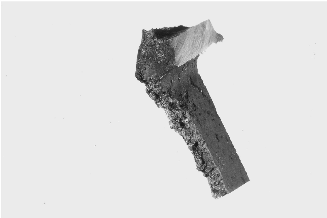
Fig. 3. Porosity in a failed bronze impeller.
