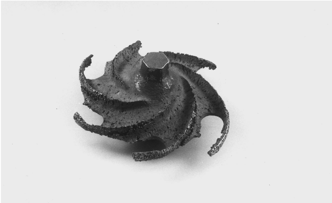
Fig. 7. Cavitation failure of cast 316 type stainless steel impeller.
