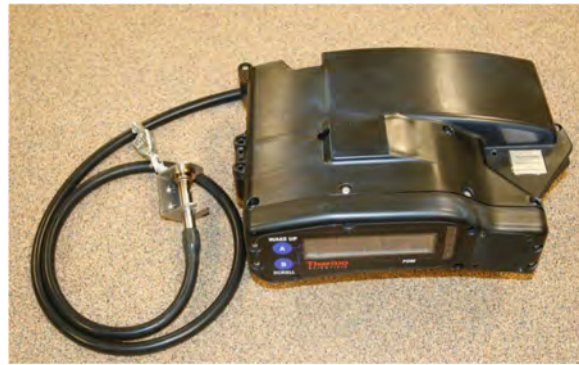
FIGURE 4-8 CPDM (PDM3700) with sampling inlet line designed to be clipped to the miner's lapel or other clothing within the miner's personal breathing zone. SOURCE: Thermo Fisher Scientific, 2016. Reprinted with permission; 2016, Thermo Fisher Scientific.
