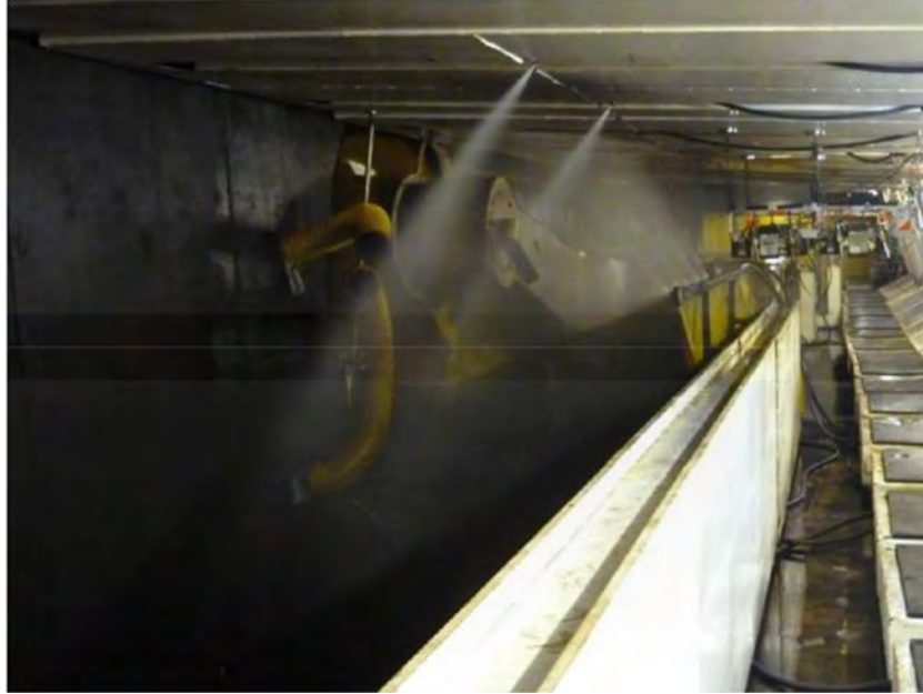
FIGURE F-7 Shields equipped with water sprays. SOURCE: Matetic, 2017.
