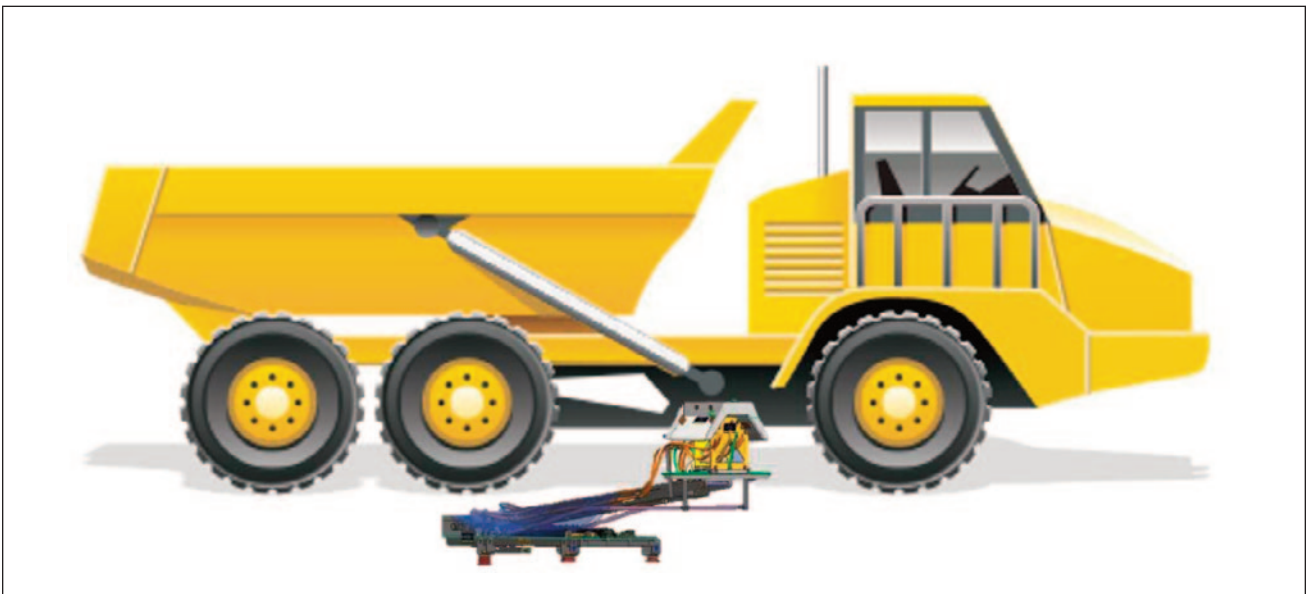
Figure 21. Underbody Charging Using a Bottom-Up Pantograph
