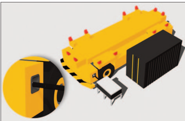
Figure 22. Automated Enclosed Pin and Socket Charging Interface
