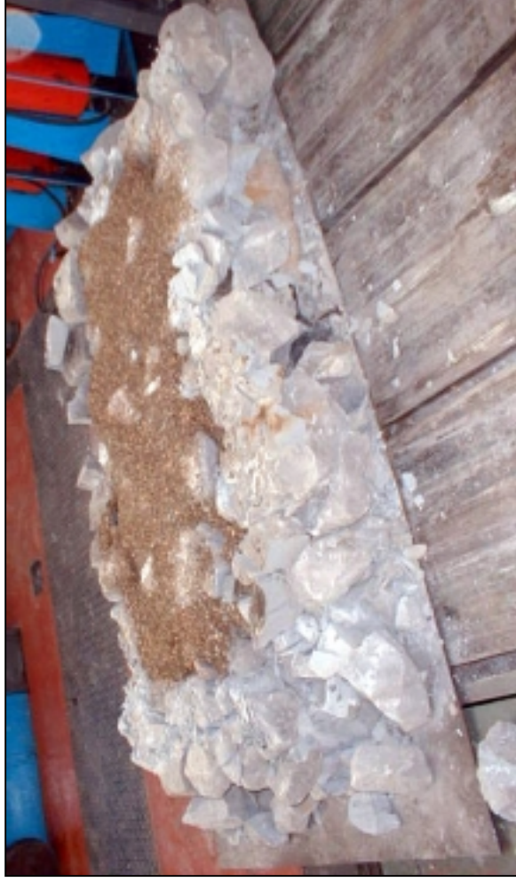
Stone packs after loading showing displaced / crushed outer wall
