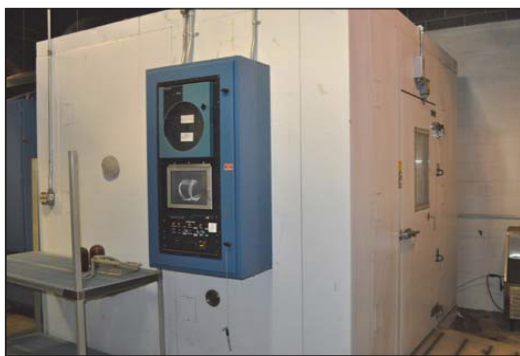
Figure 2-12. Outside view of NIOSH Environmental Conditioning Chamber
