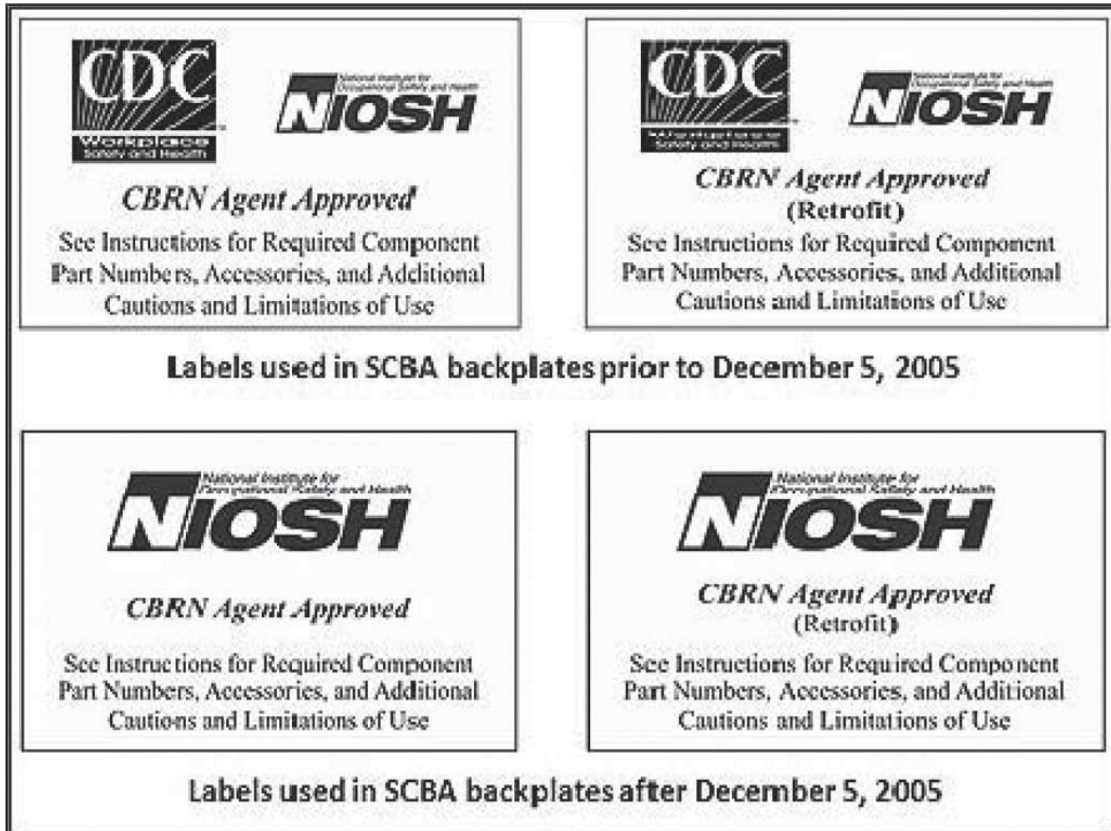
Figure 3-5. NIOSH “CBRN Agent Approved” Label (adhesive) for new and retrofitted CBRN SCBA
