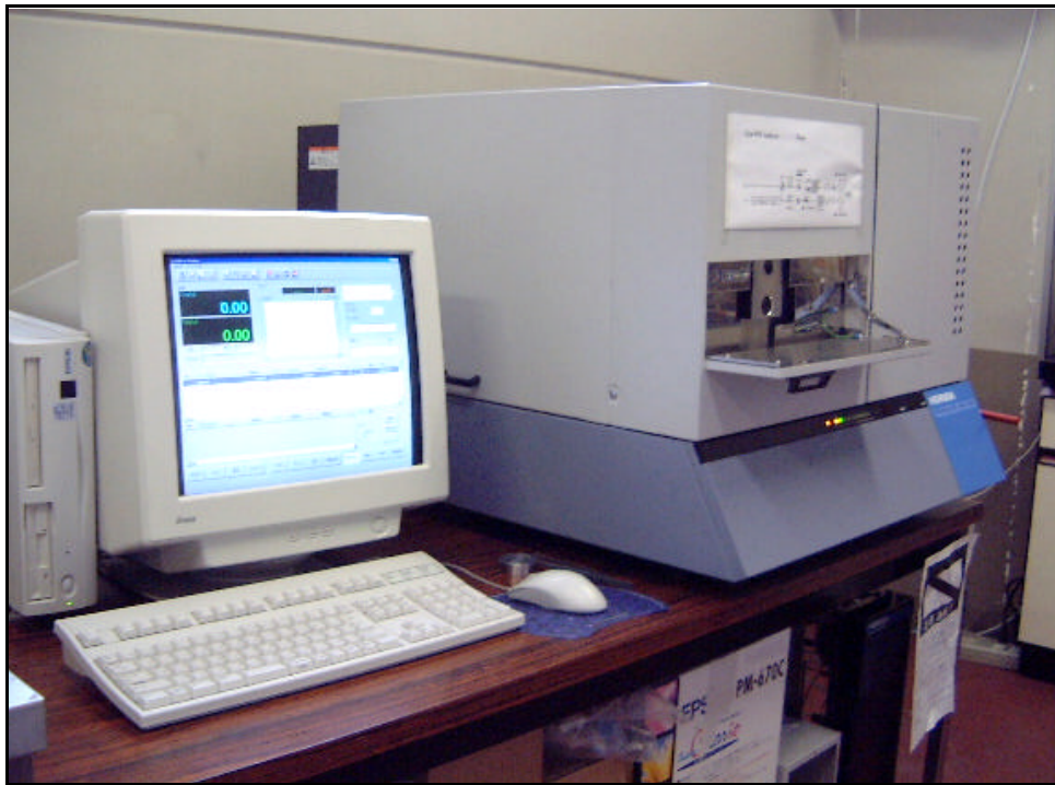
Figure 4.3.1.1: Horiba MEXA-1379PM elemental carbon analyser (Courtesy of the Engine Measurement Division, Horiba).
