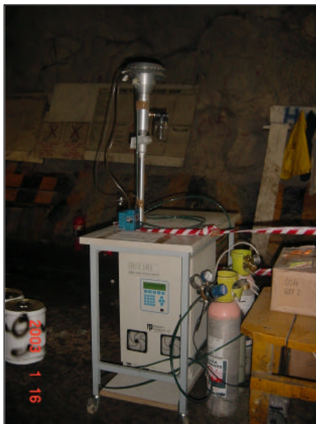
Figure 4.3.2.1: The R&P Series 5400 Ambient Carbon Particulate Monitor in place for sampling and analysis in a goldmine.
