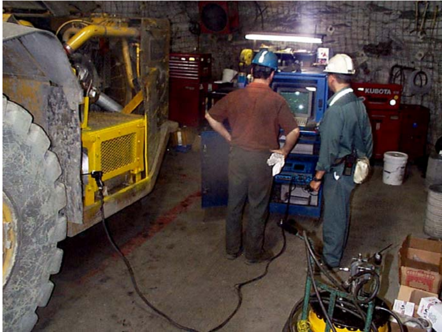
Figure 5. UGAS/ECOM direct exhaust sampling
