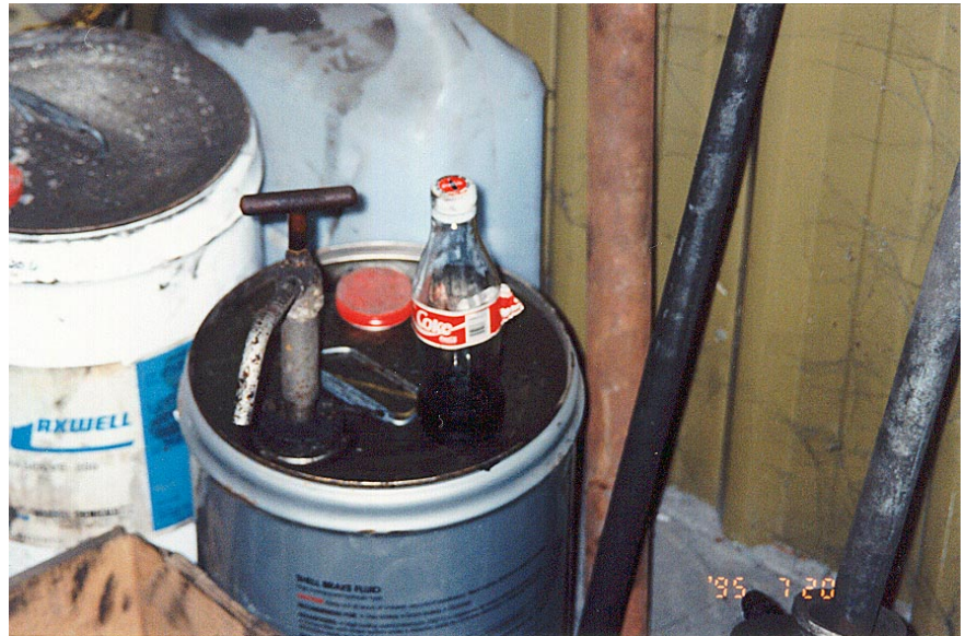
FIGURE 4-04b(VI) INCORRECT USE OF FOODSTUFF CONTAINERS
