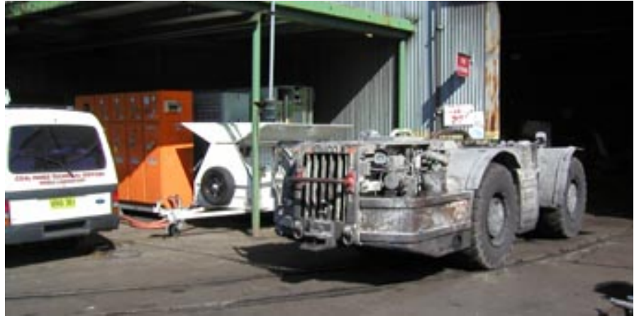
FIGURE 6-03a(VI) R&P SERIES 5100 ANALYSER AND MOBILE GAS LABORATORY ON-SITE DURING TESTING OF AN EIMCO LHD
