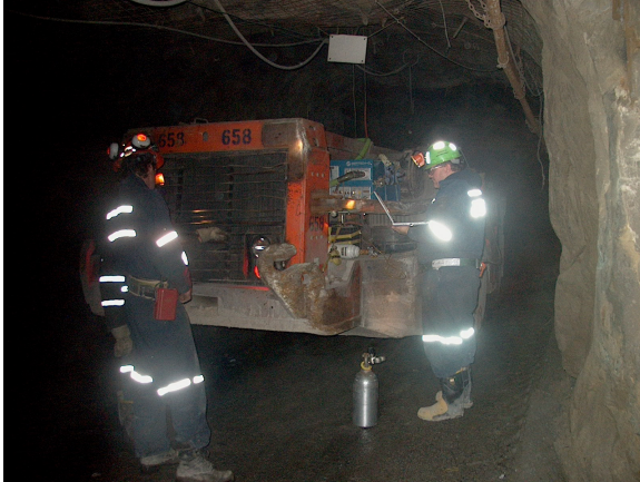
Figure 10: Technicians calibrating the SEMTECH-D analyzer
