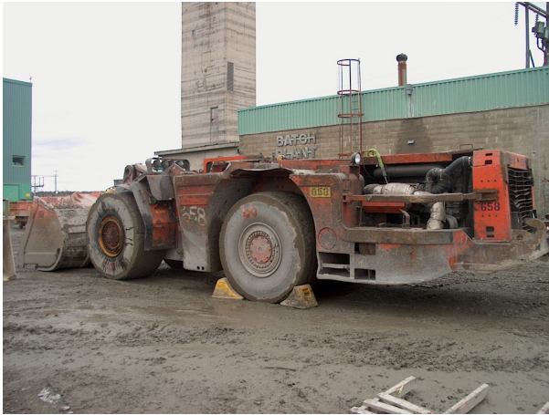
Figure 8: Toro Tamrock load-haul-dump (LHD) vehicle.
