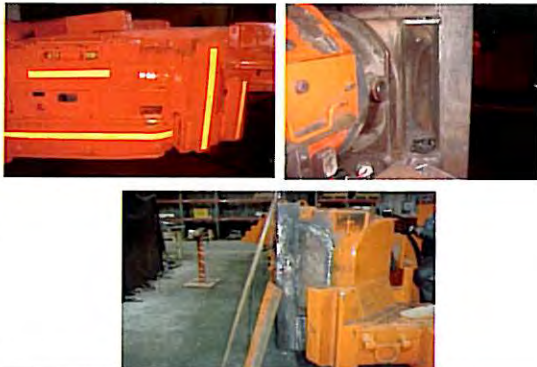
Scrubber off-side air discharge
