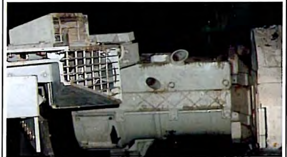
Shearer headgate end spray bar
