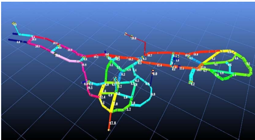
Figure 6.11. Ventsim model simulation using the West Booster and Main fans
