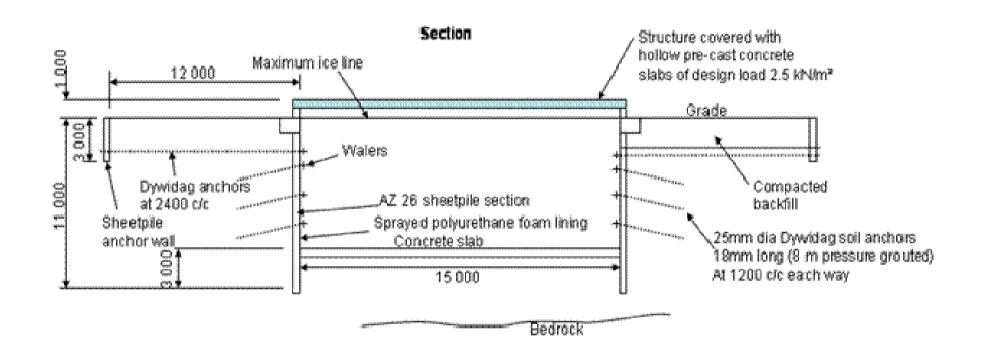
At a similar mine (climate and location), an open pit had a potential ice storage volume of about 500 000 t with an equivalent cooling capacity of just over 30 MWR. The cost was about two thirds that of a conventional plant.
