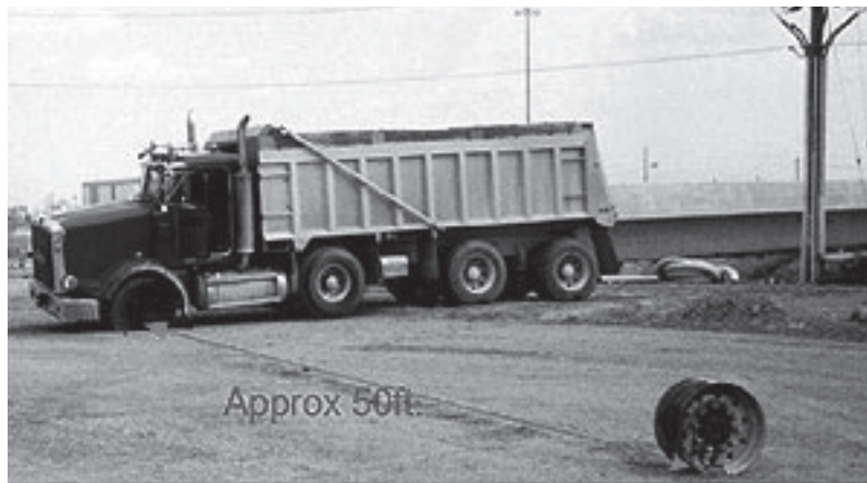
Truck tire exploded after bed contacted overhead power conductor.
