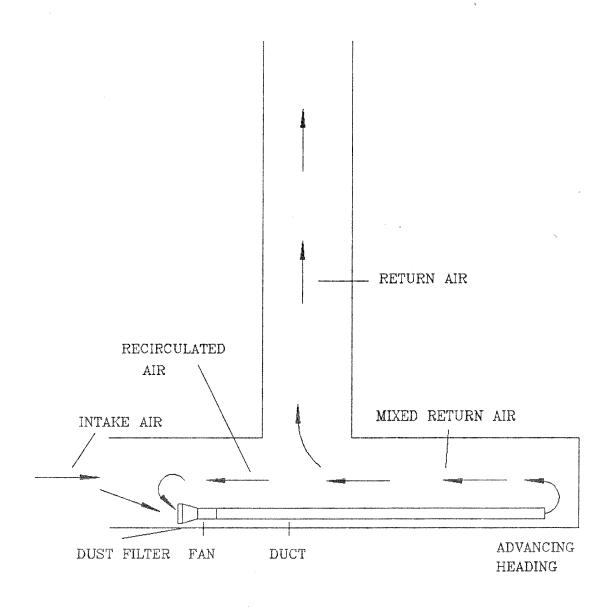
FIGURE 1. SIMPLIFIED CONTROLLED AUXILIARY RECIRCULATION VENTILATION SYSTEM
