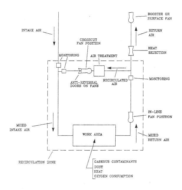
FIGURE 2. CONTROLLED DISTRICT RECIRCULATION VENTILATION SYSTEM
