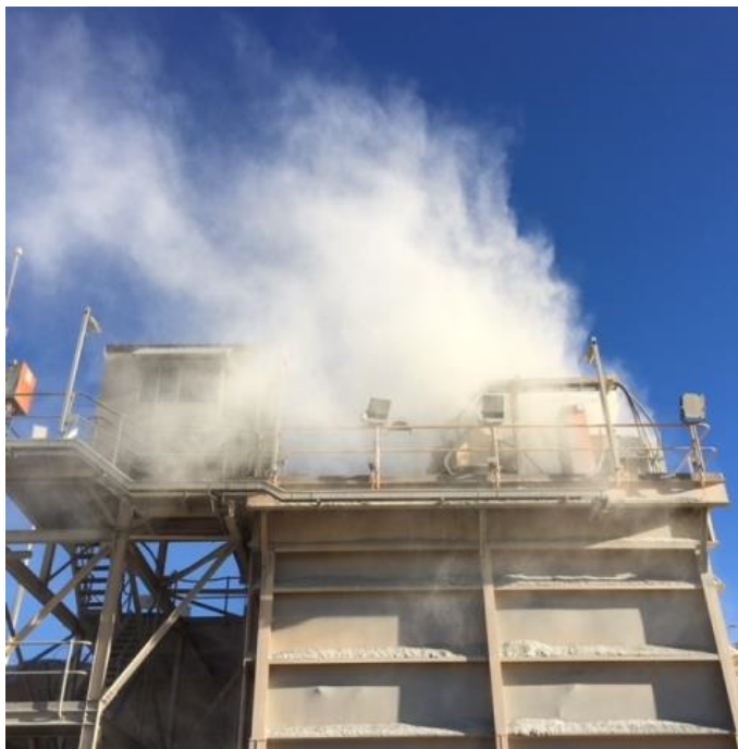
Excessive dust emission at a primary crusher hopper
