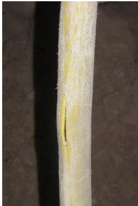
Figure 5 - Photo of grout hose showing a split, abrasions, and fine fibers.
