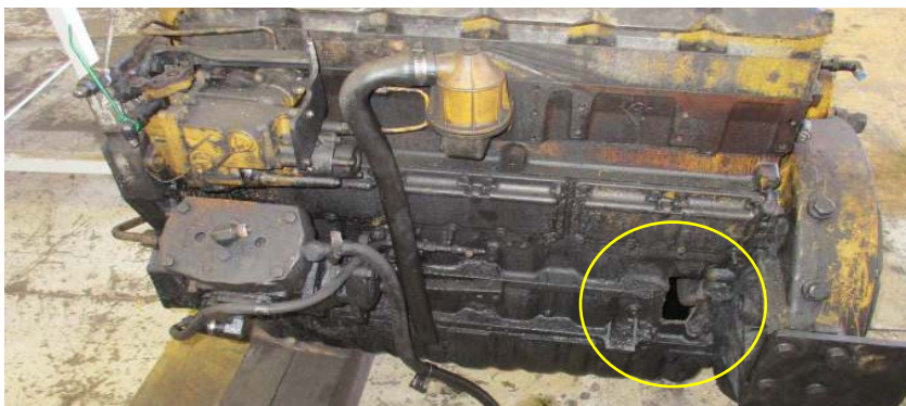
Figure 1: The hole in left rear of cylinder block (circled below) after the parts were ejected from it.
