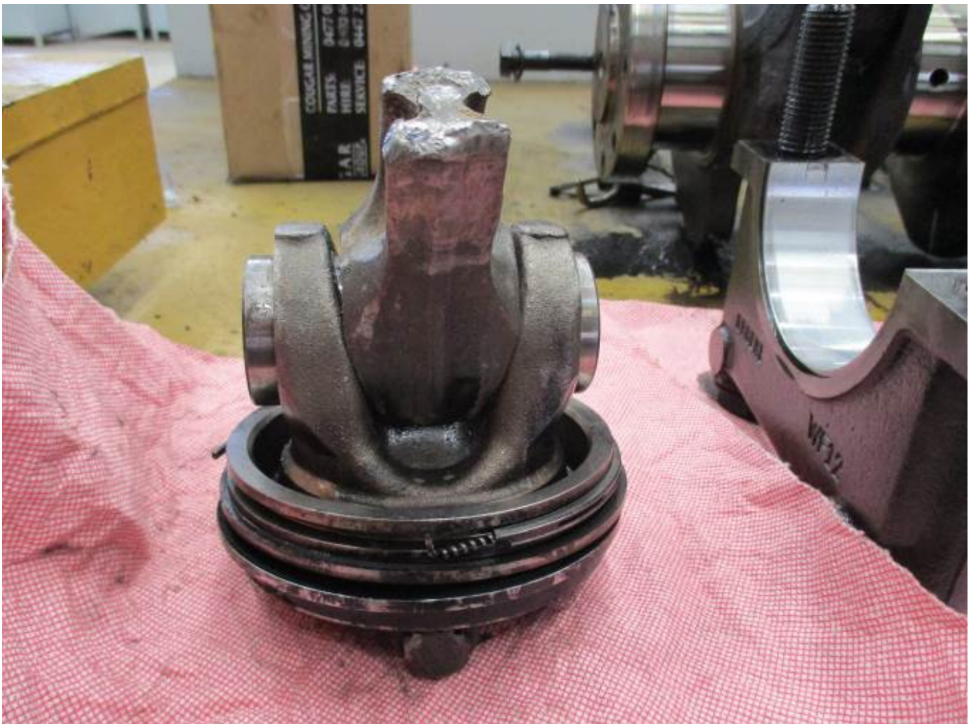
Figure 12: Piston and wrist pin with remainder of conrod attached (other part never found).
