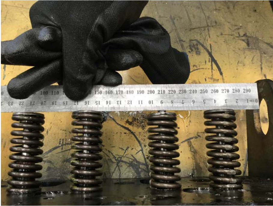
Figure 5: Valve second from left shorter than others due to bent shaft.
