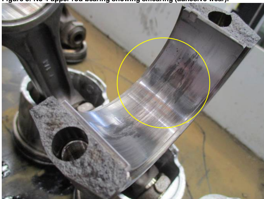
Figure 8: No 4 upper rod bearing showing smearing (adhesive wear).
