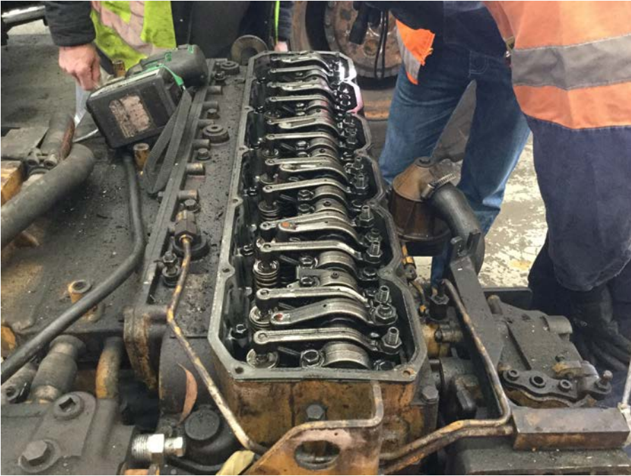
Figure 3: Rocker cover removed to access valves and fuel injectors.
