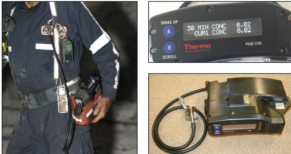
Figure 1 MSHA respirable dust rule - Phase II continuous personal dust monitor
