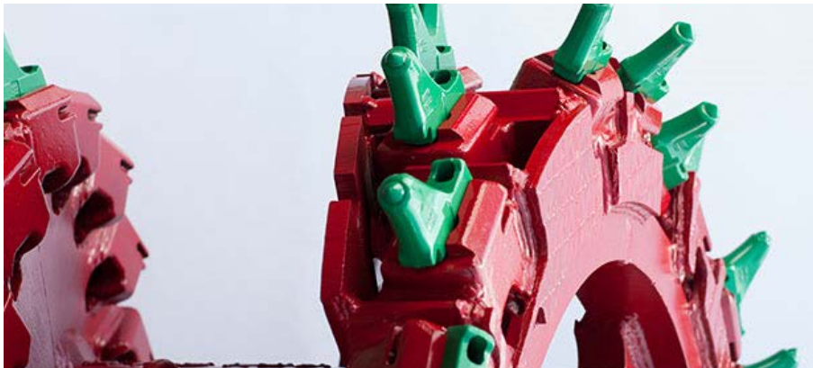
Figure 19: Shearer drum fitted with Radial picks
