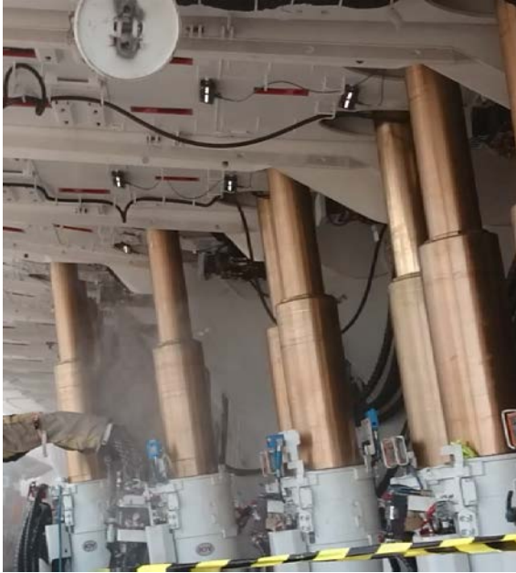
Figure 8: Leg sprays activating during LAS cycle
