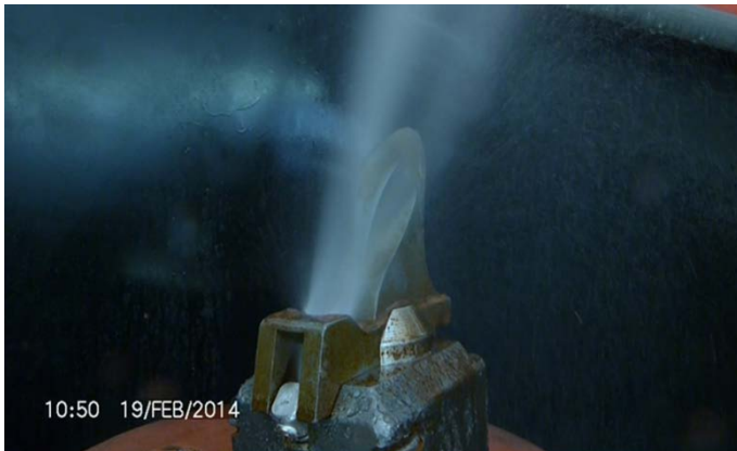
Figure 15: Back flushing pick spray
