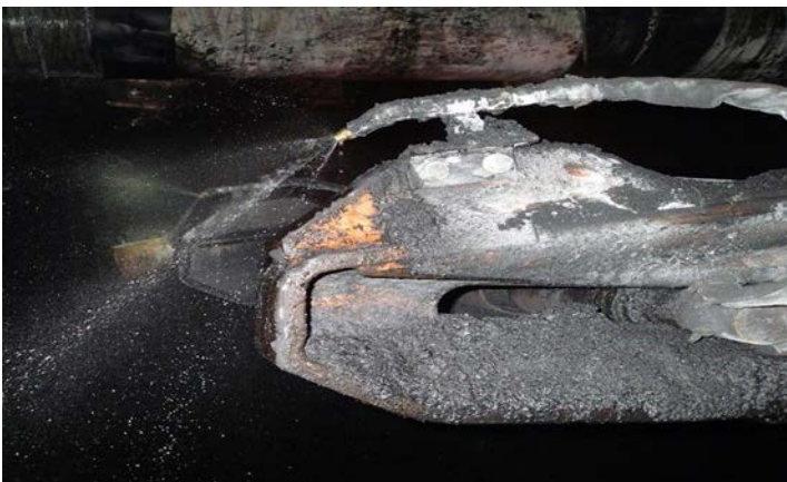
Figure 29: Single spray located on the tail of the Continuous miner.
