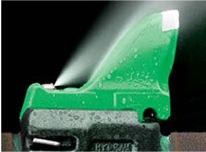
Figure 14: Back flushing pick spray
