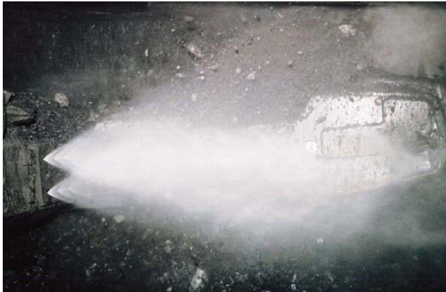
Figure 22: Side sprays on Tailgate ranging arm
