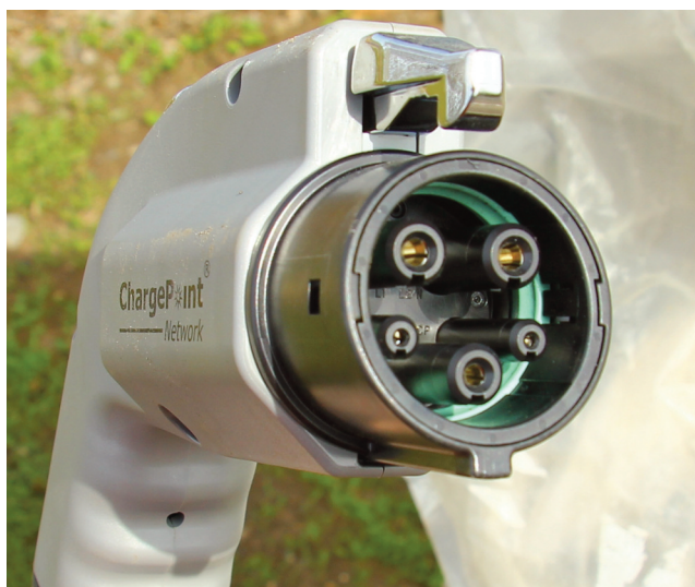
Figure 2. SAE J1772 Connector (Hicks, 2012)
