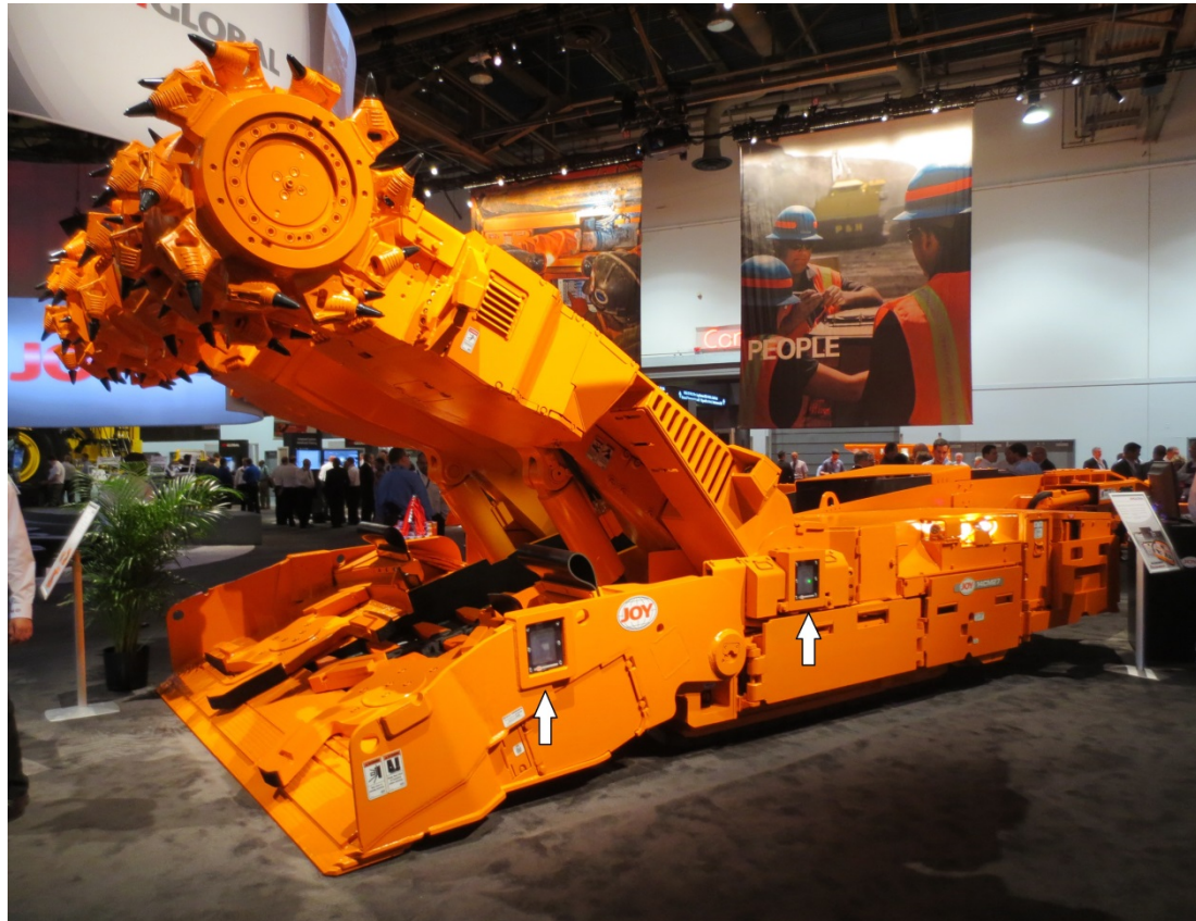
JOY Continuous Miner 12CM with a Matrix M3-1000 Proximity Detection System, at Las Vegas Mining Show in September 2012. (Picture: N. Sifferlinger)
