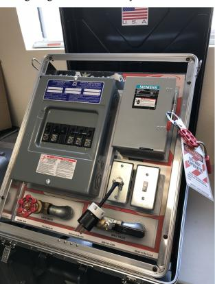
But there's more! We recently received two LOTO panels (pictured left). Each of these portable units include a variety circuit breakers and valves to practice and test your skills in LOTO procedures. We've added a supply of padlocks, hasps and some additional lock-out devices so that we can work several scenarios including locking out multiple devices and multiple people locking out on one or more devices.
