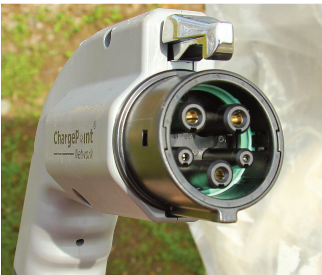
Figure 2. SAE J1772 Connector (Hicks, 2012)
