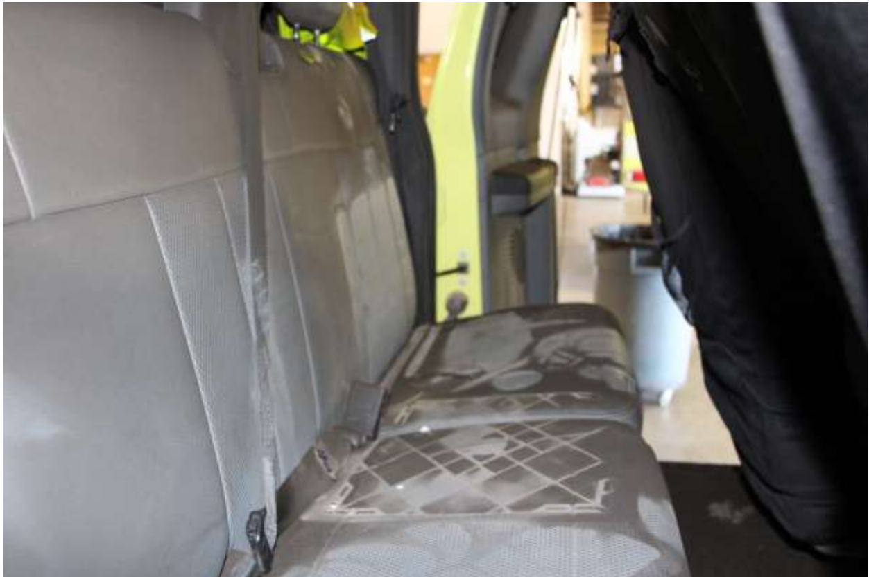
Smoke damage to back seat of cab.
