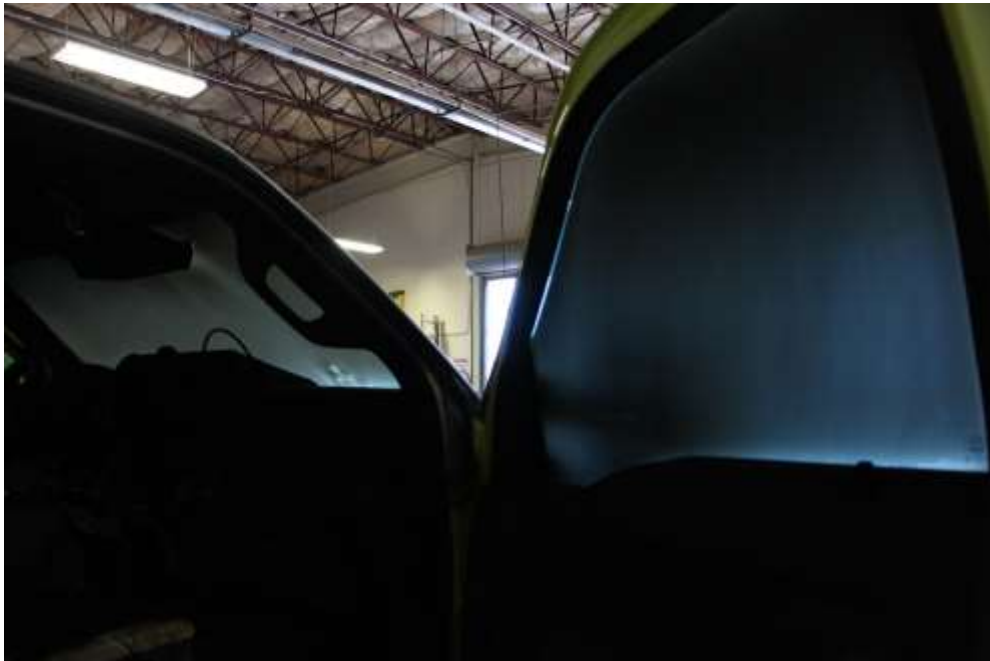
Cab windows blackened with smoke.
