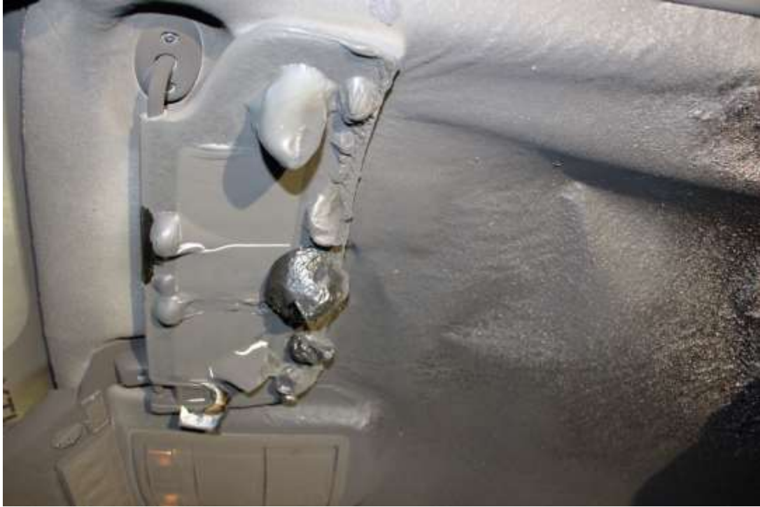
Head damage to driver's visor components.
