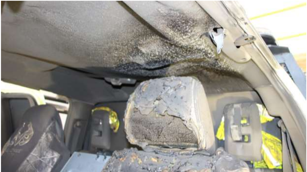
Heat damage to the headliner of the cab.
