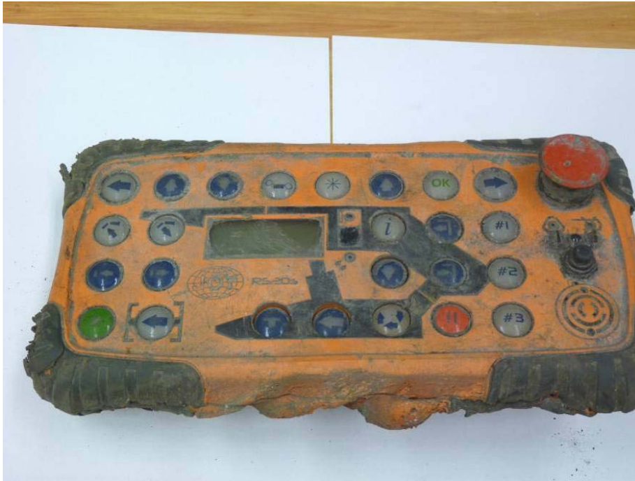
Figure 16: Joy Mimic Unit IECEx TSA 06.0029X located chock 158 LW1 top of box Photograph by Tim Flowers 24 November 2011
