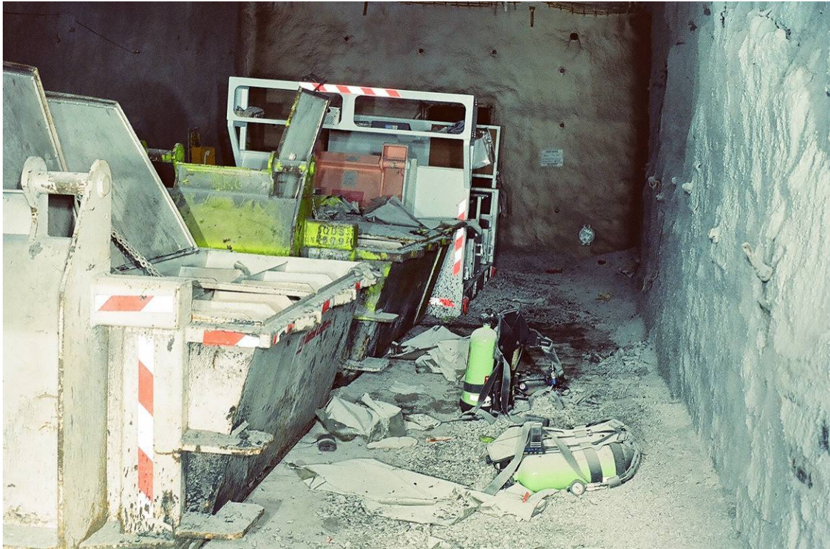
Figure 34: Photo of the two discarded CABA units as found in the crib room
