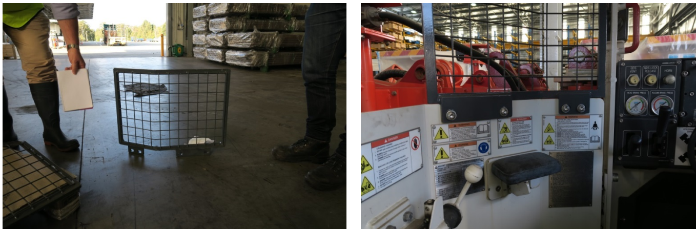
Figure 20: Guarding before and after installation.
