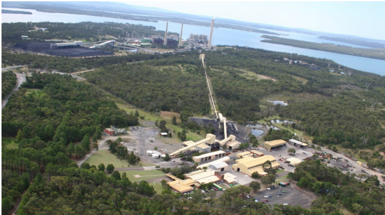
Figure 2: Mannering Colliery surface facilities and conveyor (Vales Point Power Station in background).
