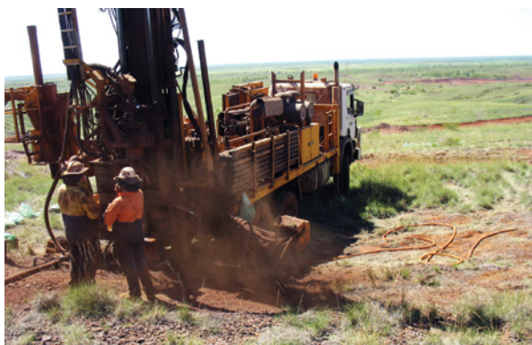
RC wet drilling (water injection)
