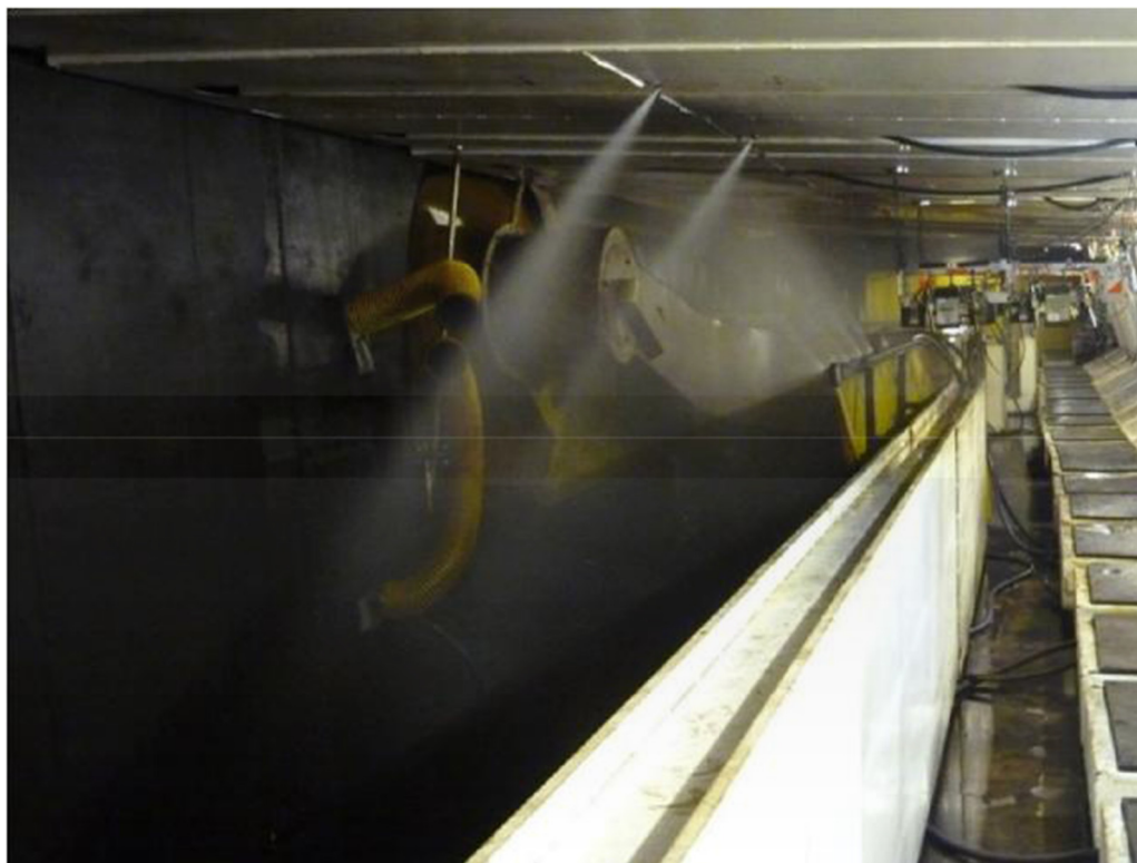
FIGURE F-13 Shields equipped with water sprays. SOURCE: Matetic, 2017.
