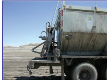
Hand rails moved closer to ladder
