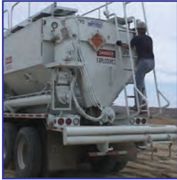
Hand rails not properly located
