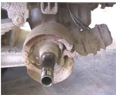
Brake pads worn off
